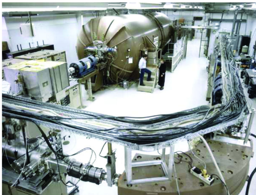
Figure 2. HVEE-FN AMS system at LLNL.
